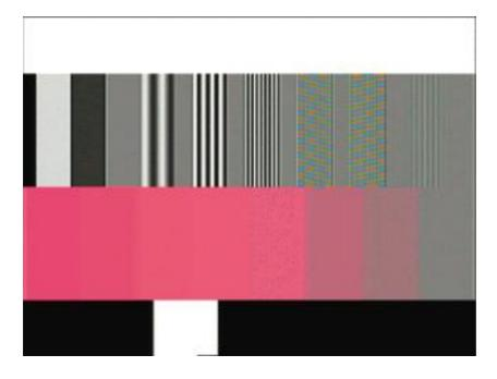
VCR 2 pattern shown, is a combined test pattern divided into three horizontal bars.
